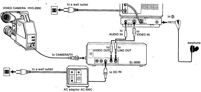
While recording the picture and sound, the controls on the receiver can be adjusted independently of the recording signal.
